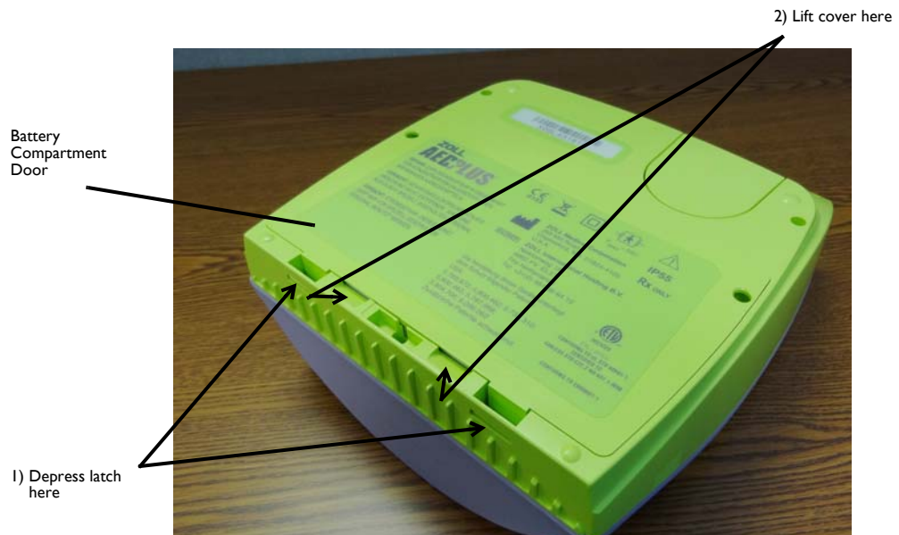
Figure 7: Removing the Battery Compartment Door
